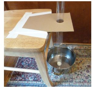
holder for tube, made from a piece of cardboard
