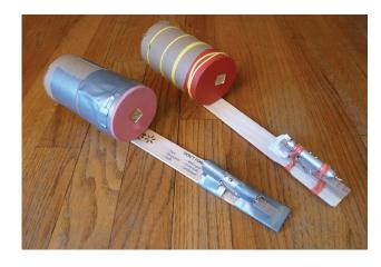
The sound vibrations of your voice make the stretched balloon vibrate. The mirror stuck to the balloon will also vibrate as a result. The laser pointer bounces off the mirror and lets you see how the mirror is moving. Thus, the sound of your voice will make the laser pointer create a pattern on the wall.
