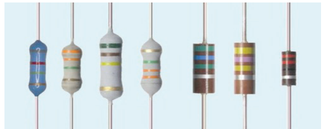
Resistors like these are used in many electronic devices today. The bands of color are codes that give information about the resistor, including how many Ohms it is.
