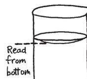
the bottom of the meniscus (the low point) not from where the water hits the sides of the cylinder.)
